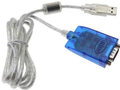
[GM-485422](#) is a universal USB to RS-485 or RS-422 converter that has no need for an external power supply. Compatible with USB, RS-422, and RS-485 standards, the GM-485422 is capable of performing the conversion from single-ended USB signal into balance differenced signal of RS-422 or RS-485. Quick state-of-the-art transient voltage suppressor (TVS) and discharge tubes are adopted to protect the RS-422 and RS-485 interfaces.
