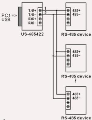
3. Half duplex connection between GM-485422 interface converters
