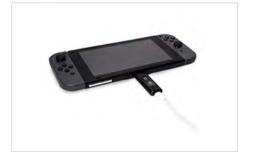
The Gearmo GM-TCPM-OLED Power delivery tester is super portable and a great tool for measuring voltage and amperage on the tech bench. The Type-C Power Meter is very easy to use. Plug the male end into the device and your power input to the female end. It is great for new USB Type-C Power Hungry devices. Data transmission is not affected by this device and uses USB 3.1 Gen1 specifications at 5Gbps speeds.
