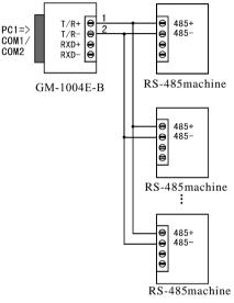
3.GM-1004E-B half-duplex communication connect between interface converter
