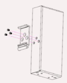
Insert the top of the DIN Rail Clip onto the DIN Rail Track, then gently push the bottom of the hub to secure it to the DIN Rail Track.
