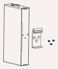
▶ Insert the top of the DIN Rail Clip onto the DIN Rail Track, then gently push the bottom of the hub to secure it to the DIN Rail Track.
