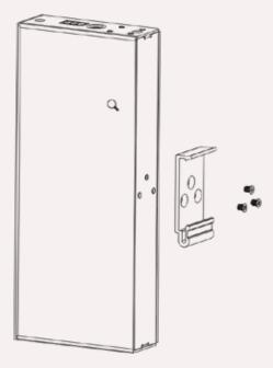
▶ Insert the top of the DIN Rail Clip onto the DIN Rail Track, then gently push the bottom of the hub to secure it to the DIN Rail Track.
